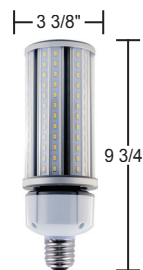
LCE39-54C-T5 Type 5 LED Lamp 54Watt, 4000K, 7290lm Replaces up to 250W MH 360° Beam Angle
