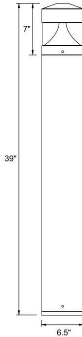
Wave Lighting's C200BC Bollard adds a modern look to any pathway. This fixture is available LED and its industrial strength features make it ETL listed and suitable for wet locations. Wave Lighting's C200BC is designed for low mounting in reinforced concrete (by others), hardware and template is included.
