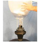
Reach into the enclosure and turn the Dark Sky Reflector so the bottom (widest part) is down toward the opening of the enclosure.
