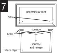
ATTACH FIXTURE ROOF TO FIXTURE HOUSING. Squeeze cage as shown. Position holes on side of cage over corresponding pins on underside of roof. Release cage - pins will snap into position.
