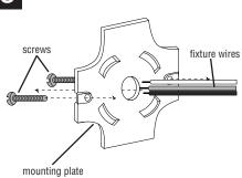
Thread the one inch long screws into the mounting plate and feed the fixture wires through the hole in the center of the mounting plate.
