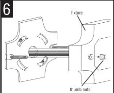
Position fixture over fixture mounting screws and secure with provided thumbs nuts.
