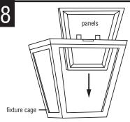
BEFORE SNAPPING HOUSING SHUT, install plastic panels, textured or beveled side out, by sliding panels down cage in slots on inside of cage. Make sure panels are all the way down into seats in cage
