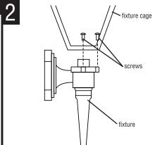
FASTEN THE CAGE to the fixture with the 3 screws provided.
