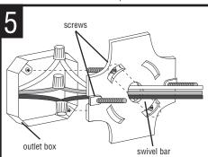
Attach swivel bar to outlet box with two 8-32 screws (not provided). These screws should be inserted through appropriate rectangular opening in plate and into swivel bar. Tighten screws.
