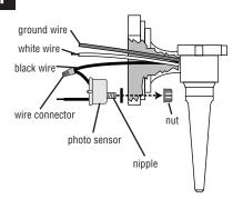
Insert nipple through hole in fixture base. Thread nut onto nipple. Connect black wire from fixture to one of the black wires from photo sensor with wire connector provided.
