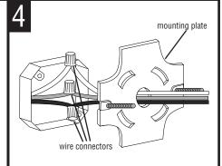
CONNECT THE WIRES. NOTE: Attach black fixture wire to black supply wire, white fixture wire to white supply wire. Do not mix them up. Use approved wire connectors (not provided). Connect bare fixture ground wire to ground wire from outlet box. NEVER CONNECT GROUND WIRE TO BLACK OR WHITE POWER SUPPLY WIRES.
