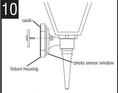
NOTE: Fixture MUST be caulked with an acrylic caulk where fixture housing meets mounting surface. This provides a water tight seal when fixture is installed.
