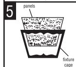
install front and rear plastic panels first, OF CAGE. Rotate free end of cage up to textured side out, then drop in side the housing and snap into place. panels.
