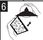
BEFORE SNAPPING HOUSING SHUT, HOLD LEFT SIDE PANEL AGAINST SIDE NOTE: Fixture MUST be caulked with an install front and rear plastic panels first, OF CAGE. Rotate free end of cage up to acrylic caulk where fixture housing meets
