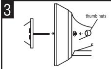
POSITION THE FIXTURE HOUSING over the fixture mounting screws and secure in place with the thumb nuts provided.
