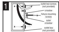
THREAD fixture mounting screws (provided) into outer cross bar. ATTACH cross bar to outlet box with outlet box screws (not provided).
