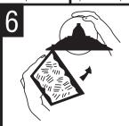
HOLD LEFT SIDE PANEL AGAINST SIDE OF CAGE. Rotate free end of cage up to the housing and snap into place. Screw bulb into socket. Be sure to use bulb with wattage no greater than specified for this fixture.
