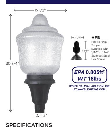
Wave Lighting's commercial product line provides safety and security for all types of applications including parks, pedestrian walkways, and parking areas. Our Post top fixtures fit on any standard 3" diameter commercial pole (sold separately). Standard 8" fitter neck acorn diffuser is easily removed by loosening 3 set screws (provided).
