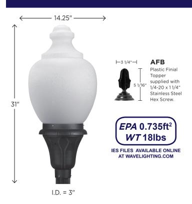
safety and security for all types of applications including parks, pedestrian walkways, and parking areas. Our Post top fixtures fit on any standard 3" diameter commercial pole (sold separately). Standard 8" fitter neck acorn diffuser is easily removed by loosening 3 set screws (provided).
