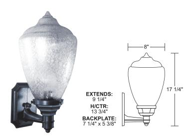
Wave Lighting's S27SC provides a level of beauty to any outdoor space. EverStone™ is a proprietary compression molded composite material that provides a level of non-corrosive durability that is unavailable in traditional metallic lighting fixtures. This fixture is available in incandescent with A19 LED lamp option and is easily relamped by unscrewing diffuser from base via 3 thumb screws. Wave Lighting's S27SC is designed for wall applications and non-corrosive mounting hardware is included.
