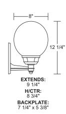
Wave Lighting's S26S provides a level of beauty to any outdoor space. EverStone™ is a proprietary compression molded composite material that provides a level of non-corrosive durability that is unavailable in traditional metallic lighting fixtures. This fixture is available in incandescent with A19 LED lamp option and is easily relamped by unscrewing diffuser from base via 3 thumb screws. Wave Lighting's S26S is designed for wall applications and non-corrosive mounting hardware is included.
