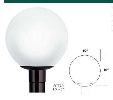
Wave Lighting's Residential Globe Fixture is ideal for any outdoor patio or walkway. This fixture is available in incandescent with A19 LED lamp option and is easily relamped via 2 screws in fitter. Wave Lighting's 10" Dia. Globe fits on a 3" diameter pole (sold separately) mounting hardware is included.
